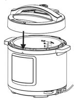
3 Rotate the lid clockwise until the ⚠ (lock symbol) on the lid aligns with the ▲ on the top front of your cooker. Make sure that the pin on the back edge of the lid is fully retracted into the lid. If the pin is visible, the lid is not closed correctly.
