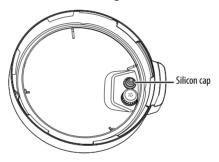
6 Put the valve protector on the inner side of the pressure release valve.
